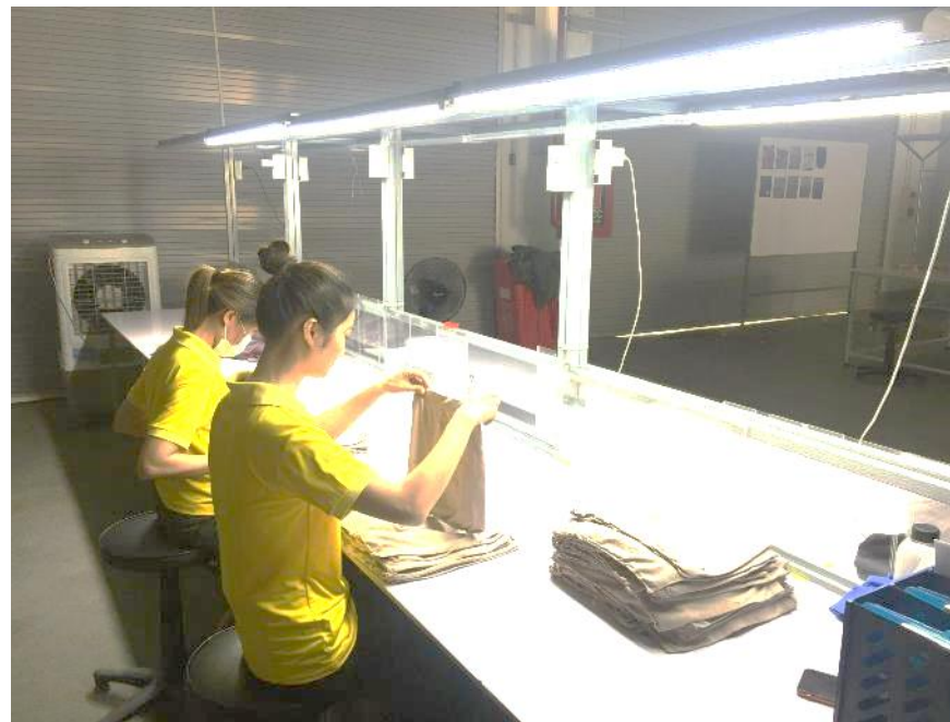
100%筒布检验 100% tube inspection before send to sewing
