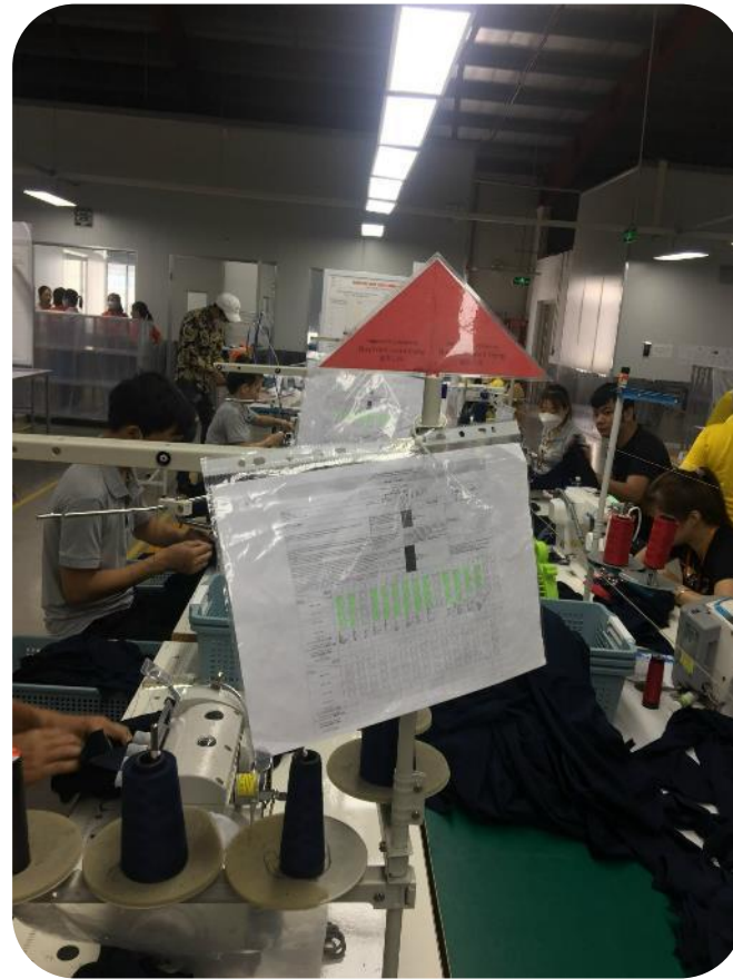
重要工序和实施的红绿灯品控系统 Key Process and implemented Traffic light system
